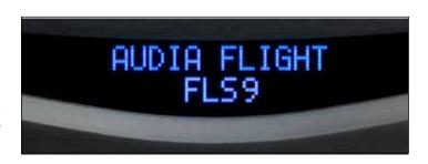
First line on display shows selected input (# 1 by default), second line shows volume level in dB of output signal (- 90 dB, by default, the lowest possible). Light in center of front panel lights in blue color, indicating operating state.
